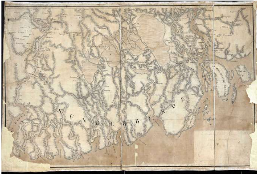
Fig. 9 The oldest topographic map of Sundarbans available at the scale of approximately 1:300,000. The map was published in 1761, and the area was surveyed in 1760. This map has geographic area and map scale, but key coordinate information is missing, making georeferencing a challenge (source: Brown, 2023)
