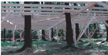
Climate change Experiment of the Bayreuth Center of Ecology and Environmental Research (BayCEER, University Bayreuth) to investigate the dynamics of soil processes under extreme meteorological conditions, meaning drying-rewetting and freezing-thawing cycles (DFG Research Group 562).
